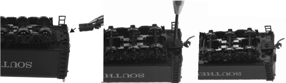
Insert the coupler (as shown) and screw into place
