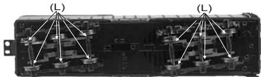
Your gearbox is properly greased at the factory and probably never needs service however, if you run excessive hours pulling heavy loads, it's a good idea to remove the 2 screws from the gearbox cover and re-grease using MTH gear grease or equivalent.
