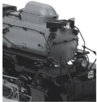
*Align the clamshell into place on top of the smoke stack*
