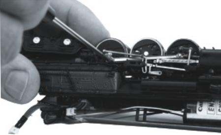
**MAKE NOTE OF THE ECCENTRIC CRANKS IN REACTION TON THE AXLE IF THE DRIVER BEING CHANGED. THE ECCENTRICS MUST BE RE-ASSEMBLED IN THE SOME POSITION.**
