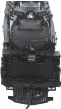
Engine Coupler Installed Front View
