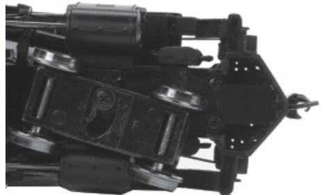
Engine Coupler Installed Underside View
