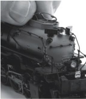
*Gently remove the folded clamshell from the top of the smoke stack*
