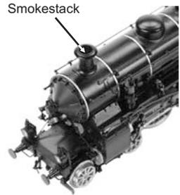
The smoke unit is controlled differently depending upon how you run your engine so, for particulars on turning it on or off or setting the output levels, check out the features and operation section. You shouldn't run your smoke unit without fluid. Doing so can cause overheating and reduce the performance and/or life of the unit. Of course, we recommend using only MTH ProtoSmoke fluid. Super Smoke and LVTS brands also work fine.
