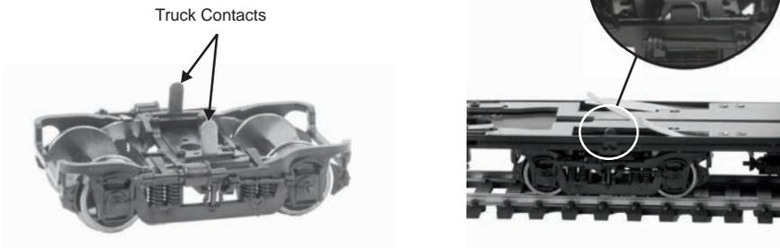
7) If you are still having problems with the car lighting up make sure the top of the contacts are bent up to make contact with the contact plates on the roof light board.
