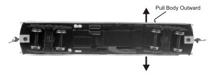
If you need to completely separate the body from the chassis simply remove the connector.
