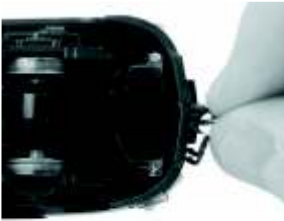
Line Up CENTER Mounting Hole In Coupler Pocket With Mounting Hole On Chassis
