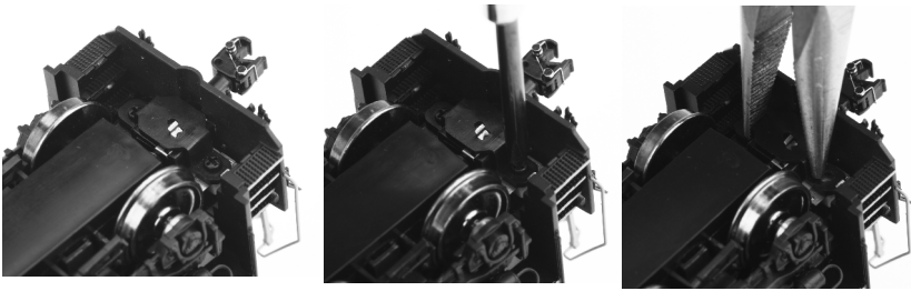
Identify & Remove Mounting Screws
