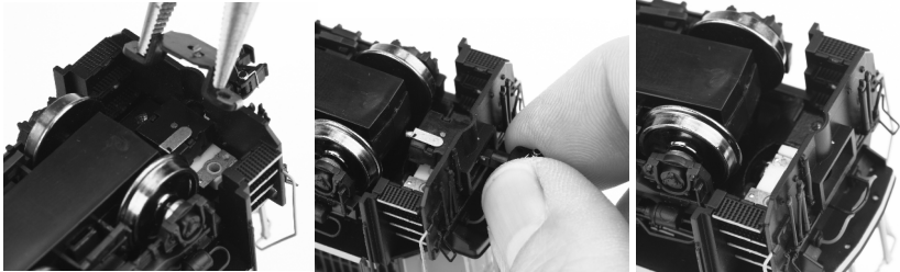
Lift Out Cover Plate & Pull Coupler Mechanism Out Through Pilot Hole
