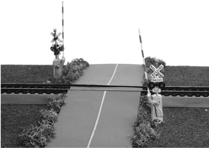
8. If you have a dimly lit room you may find that your sensors are not detecting the train. To increase the sensitivity of the sensors turn the sensitivity pot clockwise.
