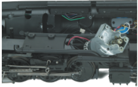
Figure 19: Lifting Motor Away From Truck Block
