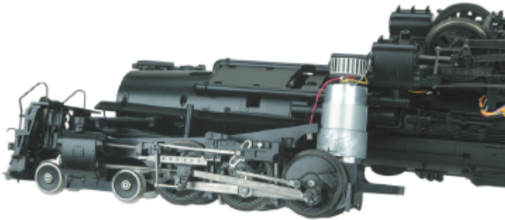
Figure 16: Turn The Chassis Over To Remove The Top Motor Mount Plate
