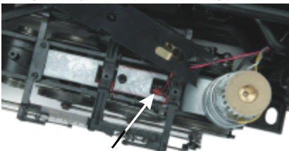
To Lift The Plate, It May Be Necessary To Unplug The Pickup Harness.
