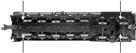
Figure: Body Mount Screw Locations
