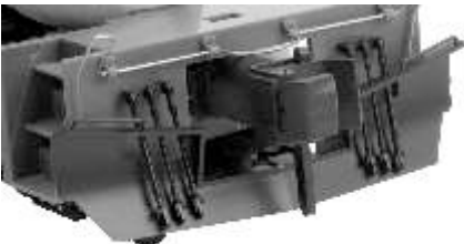
Figure: Installed Snow Plow
