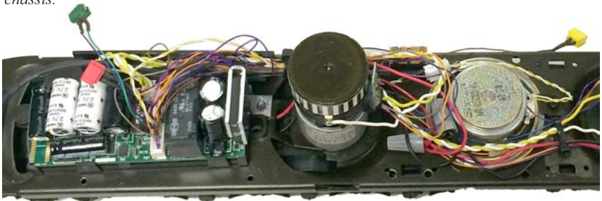
Typical component arrangement on tender floor. Note position of heat sink.
