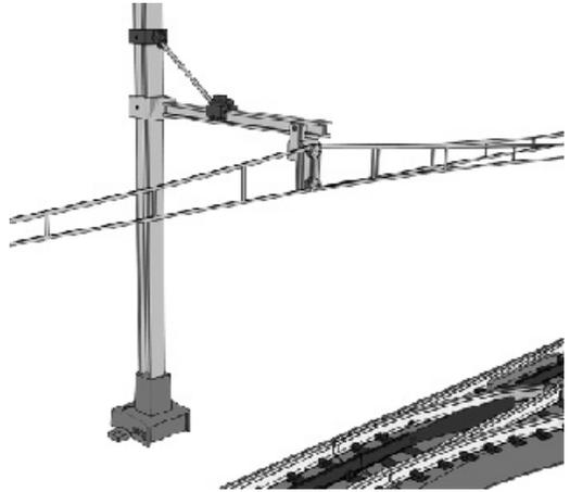
Attach three wires to the brace to wire a switch.
