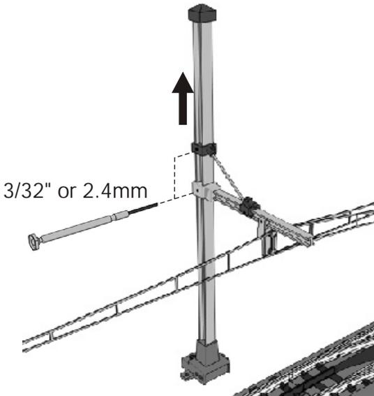
Adjust the messenger arm by turning the screws shown with a 2.4mm screw driver.
