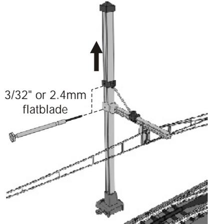
Adjust the messenger arm height by turning the screws shown with a small screwdriver.
