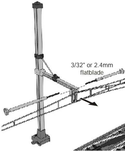
Adjust the messenger brace by turning the screws shown with a 3/32" or 2.5mm flatblade screw driver.
