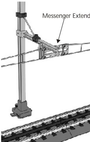
To extend the reach of one of your messenger wires, add a messenger extension plate. Attach one end of the plate to the brace and screw the wire to the appropriate holes in the other end of the plate.
