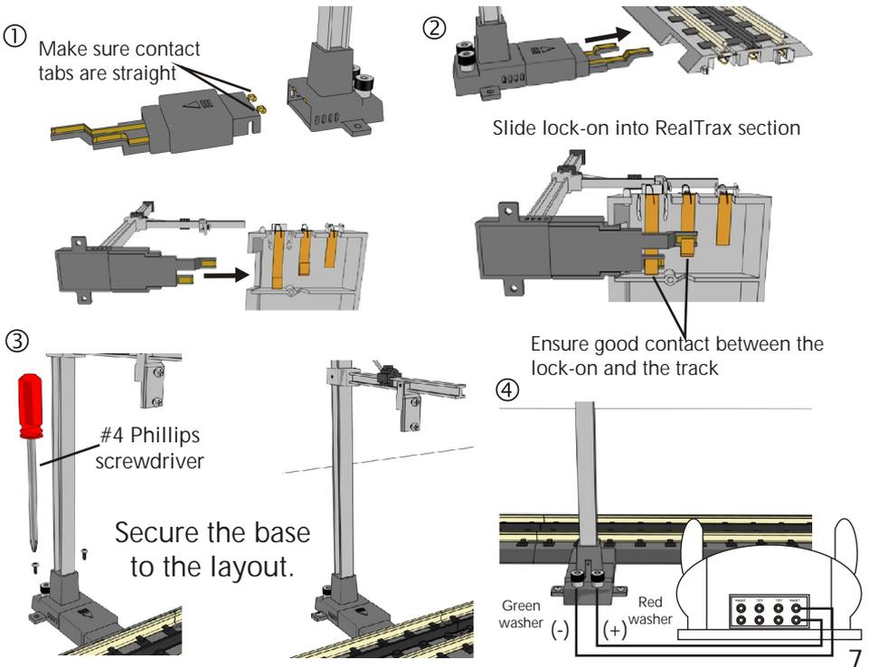
2. To allow the catenary to share existing RealTrax track power from an existing RealTrax lock-on:
