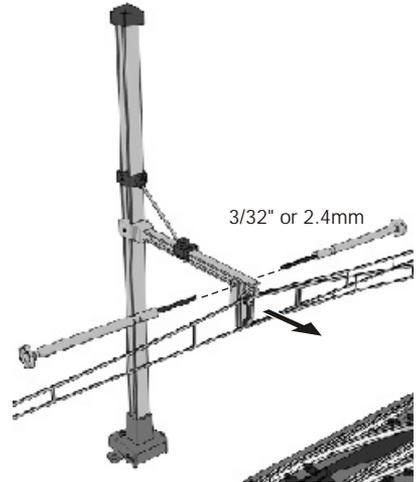
Check to make sure messenger wire always has contact with the engine's pantograph's.
