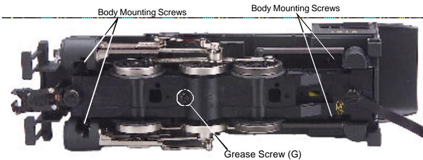
*Figure 4. Greasing Points on the Engine and Body Mounting Screws*
