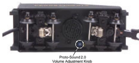
*Figure 1. Adjusting the Proto-Sound 2.0 Volume Level*
