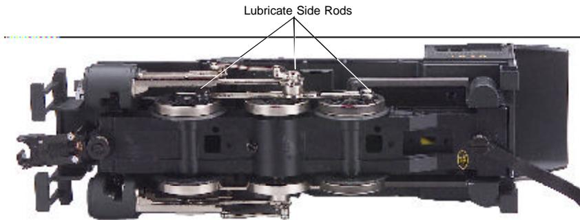
*Figure 3. Lubrication Points on the Engine*
