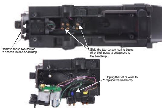
*Figure 9. Replacing the Headlight*
