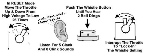
*Note: When “Whistle In Neutral” is set, the bell will only operate with a separate bell button and the whistle will not sound in neutral if the transformer throttle setting is over 11 volts. At 11 volts or higher, ProtoSounds® may arm the coil coupler for operation whenever the whistle button is pressed and the engine is in neutral.*
