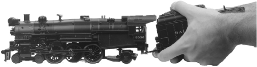
Fig. 4: Connecting Locomotive to Tender
