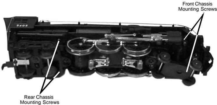
Figure 10: Removing The Boiler From The Chassis
