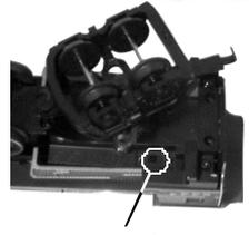
Figure 3: Smoke Unit Switch
