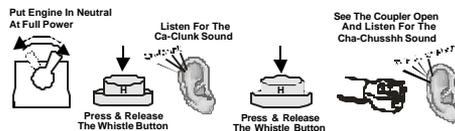
The coupler doesn't have to be fired in NEUTRAL. Once the coupler is armed it can be fired in Forward, Neutral or Reverse. However, you may find that the coupler doesn't open when firing the coupler at high speeds. Reduce the voltage setting on your transformer if this occurs and run your engine at a slower speed before firing the coupler. If the coupler continues to open erratically, try lubricating the knuckle with light oil as indicated in Fig. 5.
