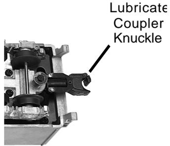
Figure 5: Lubricating The Coupler
