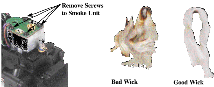
Figure 8 - Inspecting the Smoke Unit
