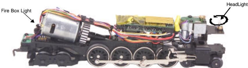
*Figure 8. Replacing the Headlight and the Fire Box Light*
