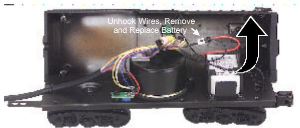
Figure 9. Replacing the Battery
