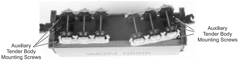
Figure 1: Removing The Auxiliary Tender Chassis
