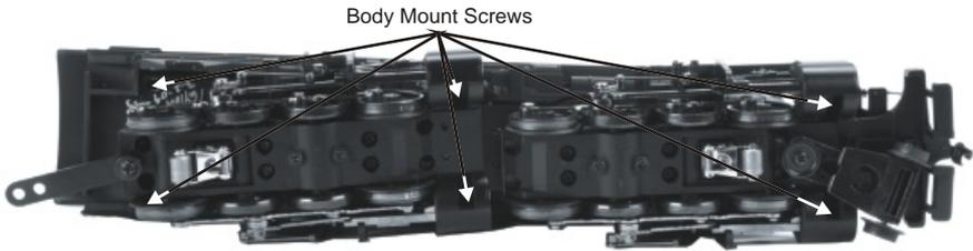
*Figure 5: Removing the body*
