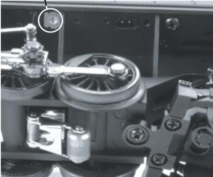
**Figure 2. NOTE:** Smoke Unit Switch is now a volume pot type control. The amount of smoke can be varied by the adjustment of the smoke control under the tender. By rotating the control, the smoke can be varied from off to full force or any amount in between.
