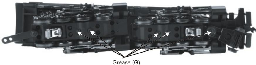
Figure 6: Motor Gearing Grease Plate Screws
