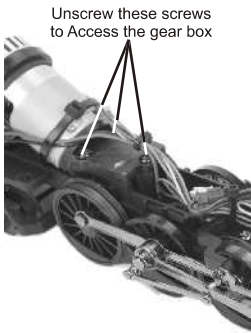
Figure 7. Motor Gearing Grease Plate Screws
