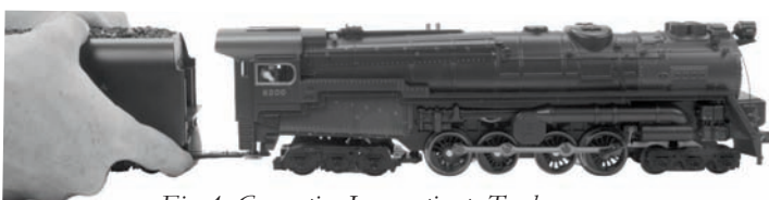
Fig. 4: Connecting Locomotive to Tender
