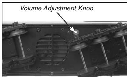
Figure 1 - Proto-Sound 2.0 Volume Adjustment Knob
