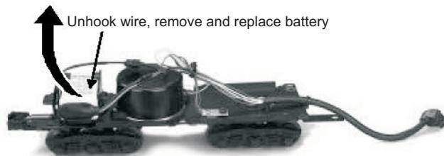
*Figure 8. Replacing the Battery*
