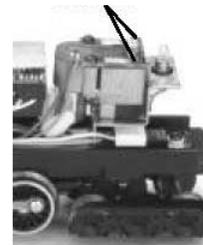
Figure 6. Smoke Unit Inspection Cover
