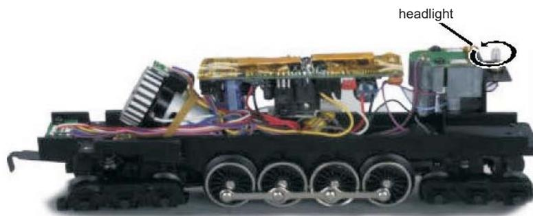
*Figure 7. Replacing the Headlight*
