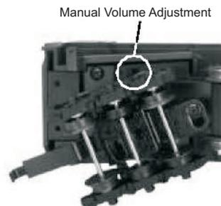
*Figure 1. Proto-Sound 2.0 Volume Adjustment Knob*
