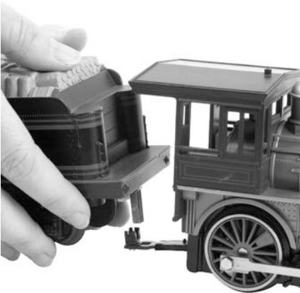
Figure: Connecting Locomotive to Tender
