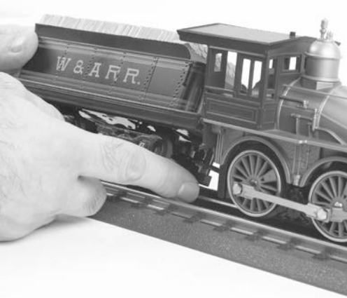
Figure: Attaching the Plastic Drawbar Holder
