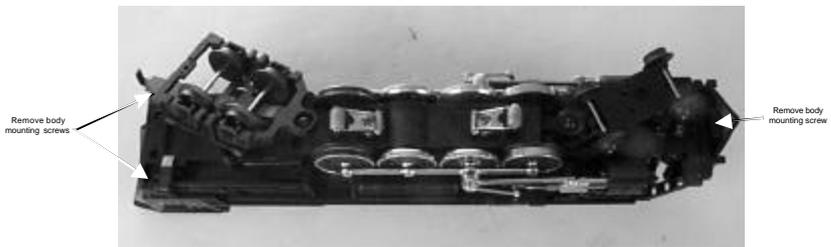
*Figure 10: Removing The Boiler From The Chassis*
