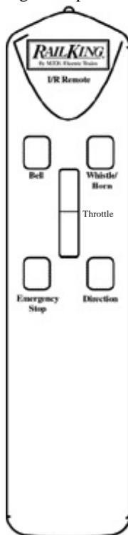
**Horn/Whistle** - To sound the horn, firmly press the Horn/Whistle button. The horn will sound for as long as you continue to depress the button. It will stop when you release the button.
