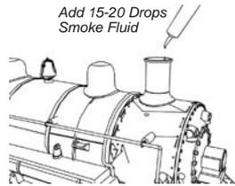
**⚠ Running the engine without a primed smoke unit may cause damage**
