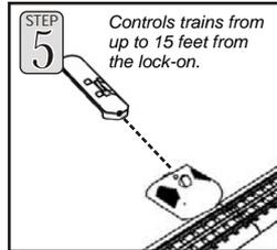
Controls trains from up to 15 feet from the lock-on.
