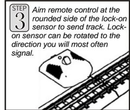
Aim remote control at the rounded side of the lock-on sensor to send track. Lock-on sensor can be rotated to the direction you will most often signal.
