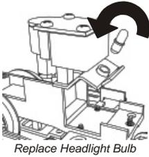
Once the locomotive boiler has been removed from its chassis, locate the bulb bracket as seen in the illustration on the right and rotate the headlight bulb counter-clockwise to remove.
