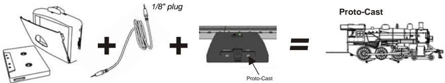
**Proto-Dispatch:** This feature allows you to broadcast your own voice through your engine's speakers. You must supply the microphone and a mini cable (1/8" plug, like that used for the headset with a portable CD/tape player) to connect your microphone to the remote lock-on.
