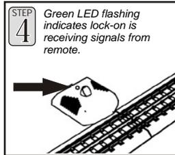
Green LED flashing indicates lock-on is receiving signals from remote.
