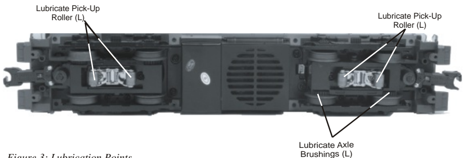
Figure 3: Lubrication Points
