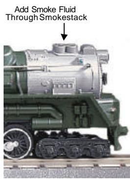
Figure 4. Add Smoke Fluid Through the Smoke Stack
