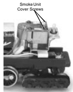
*Figure 13. Inspection Cover Screws*
