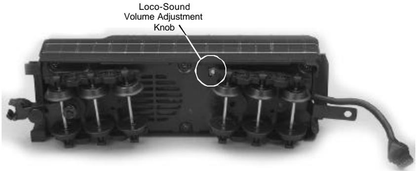
*Figure 10. Location of Loco-Sound Volume Adjustment Knob*
