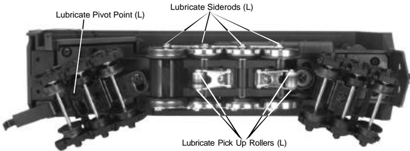
*Figure 11. Lubrication Points on the Locomotive*
