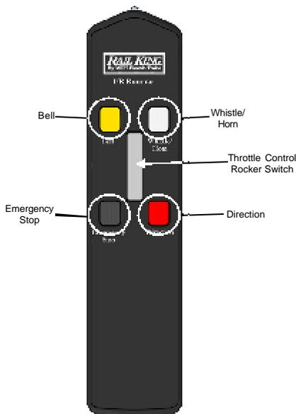
*Figure 8: Overview of the Remote controls*
