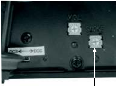
Figure 2: Smoke Unit Control Smoke Unit Control (on bottom of tender)
