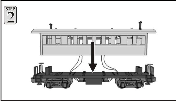
2) With the four screws removed, lower the chassis from the shell, take care not to pull the wires out.
