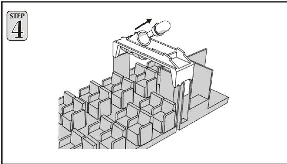
4) You can now replace the bulbs by pushing the socket up from the bulb holder and pull the bulb from its socket. Replace with a new one, and reverse the steps to reassemble the caboose.
