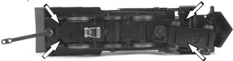
**STEP 2** Once the locomotive boiler has been removed from its chassis, locate the bulb bracket as seen in the illustration on the right and rotate the headlight bulb counter-clockwise to remove.
