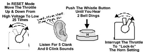
throttle off and then on again to “Lock-In” your selection. Now, whenever you are in neutral, you can blow the horn with the transformer whistle button. To reset ProtoSounds® to its original factory setting of no horn in neutral, repeat the above procedure but keep pressing the whistle button in Feature 25 until ProtoSounds® only dings once instead of twice.
