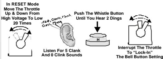
then on again to “Lock-In” the new setting. To turn the bell button function off, repeat the above procedure but keep pushing the whistle button until the computer only responds with one bell ding.
