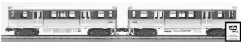
Thank you for purchasing the RailKing CTA 4-Car Subway Set. The set's durable ABS bodies and die-cast trucks are patterned and decorated after the Chicago Transit Authority cars. The cars should operate for years on any O-27 Gauge track with any compatible AC transformer (see the chart on page 28 for a list of compatible transformers) and are completely compatible with most 3-rail locomotives, rolling stock and accessories.
