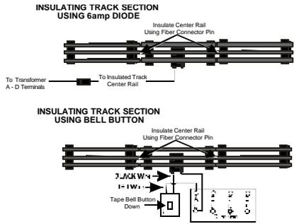
caution should be taken that not too much power is on the track or the car may pass through the insulated section before 3 seconds of negative DC was received by the ProtoSound® module. This will be obviously the case if the car's bell turns on instead of it stopping.
