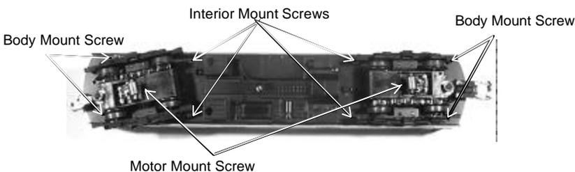
Figure 5: Removing The Body From The Chassis
