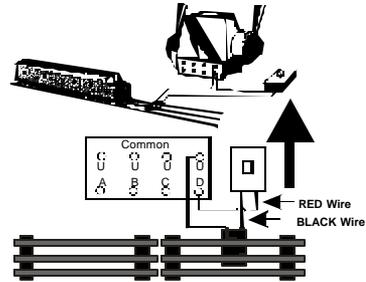
Figure 2: Wiring Up A Bell Button
