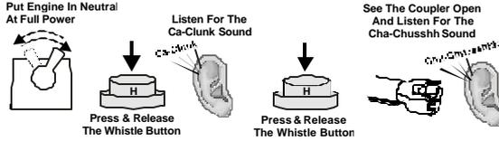
Reverse. However, you may find that the coupler doesn't open when firing the coupler at high speeds. Reduce the voltage setting on your transformer if this occurs and run your engine at a slower speed before firing the coupler. If the coupler continues to open erratically, try lubricating the knuckle with light oil as indicated in Fig. 3 on page 22.
