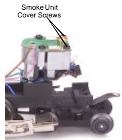
Figure 13. Inspection Cover Screws
