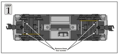
To remove the shell from the chassis, remove the four mounting screws located underneath the trucks.
