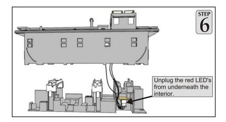
There will be two spots of hot glue holding the LEDs in place. Use a screw driver to loosen the wires from the spots of glue. Pull the LEDs back towards the inside of the shell to remove them. Replace the LEDs with a new set and use hot glue to put the wires back in place. Plug the wires back into the connector under the interior. When reassembling, the end posts of the shell must pass through the corresponding holes in the interior.
