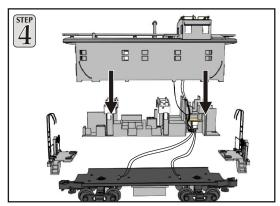
With the step platforms removed you can then lower the interior from the shell (to completely remove the body from the interior, go to Step 6 which is found on the back page).
