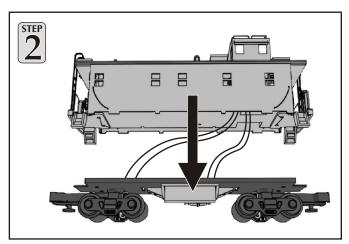
With the four screws removed, lower the chassis from the shell, take care not to pull the wires out.
