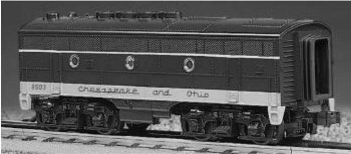
Thank you for purchasing the RailKing production of the F-3 B Unit diesel engine. The engine's durable ABS body and die-cast trucks are traditionally sized for operation on any O-27 Gauge track. The engine makes a perfect compliment for a powered Alco F-3 AA diesel engine set and is completely compatible with most 3-rail locomotives, rolling stock and accessories.
