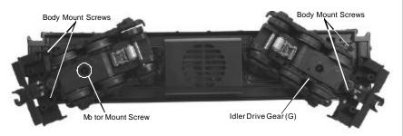
Figure 3. Lubrication Points on the Engine
