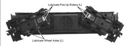
Figure 2. Lubrication Points on the Engine
