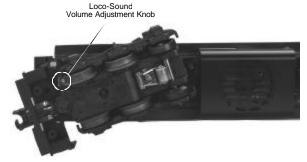
Figure 1. Location of the Loco-Sound Volume Adjustment Knob
