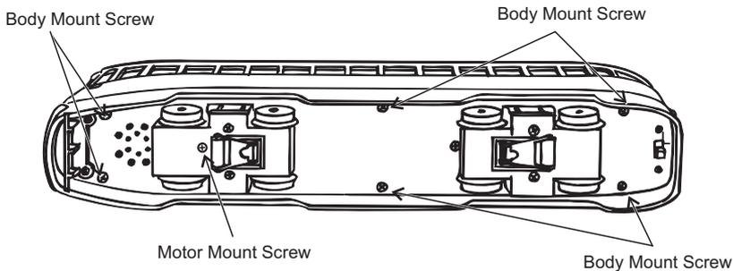
Figure 5: Removing The Body From The Chassis
