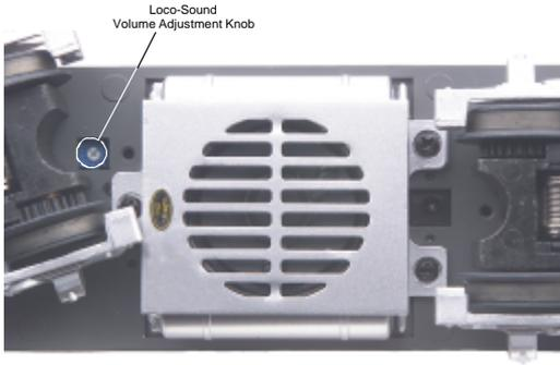
*Figure 1. Location of the Loco-Sound Volume Adjustment Knob*
