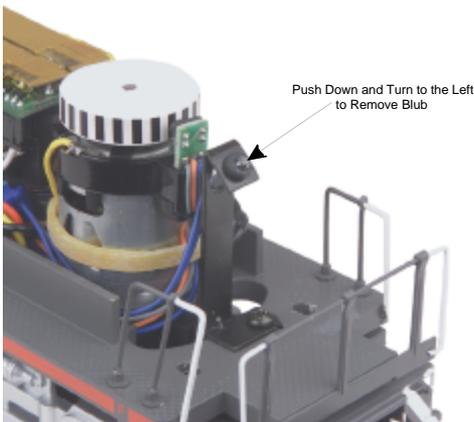
*Figure 5. Location of the headlamp in the Engine.*
