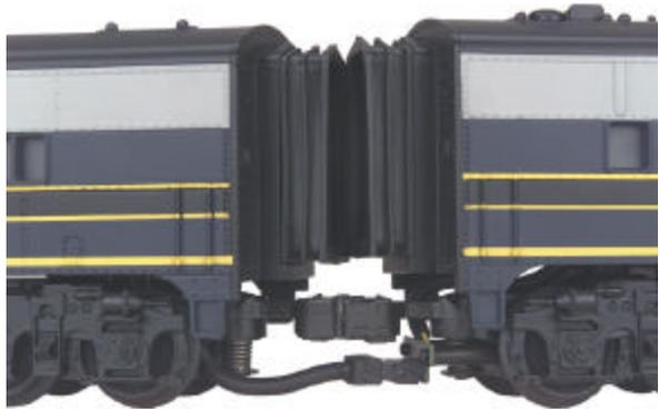
*Figure 2: Connecting the Proto-Sound Harness*
