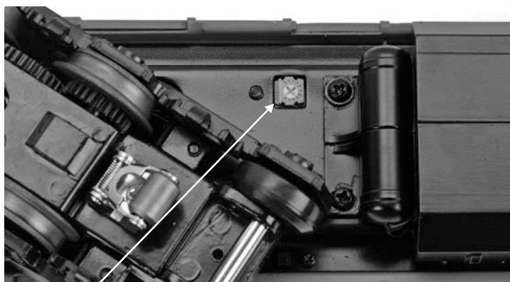
Smoke Unit Control
