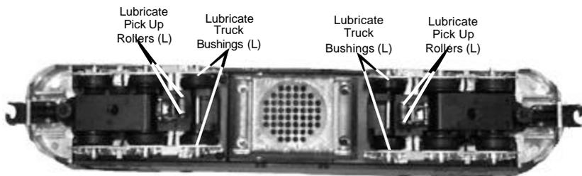
Figure 7: Lubricating The Truck
