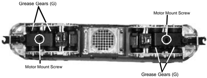
Figure 8: Greasing The Power Trucks
