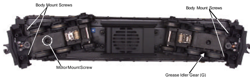
Figure 3. Body Mount Screws and Greasing Points.
