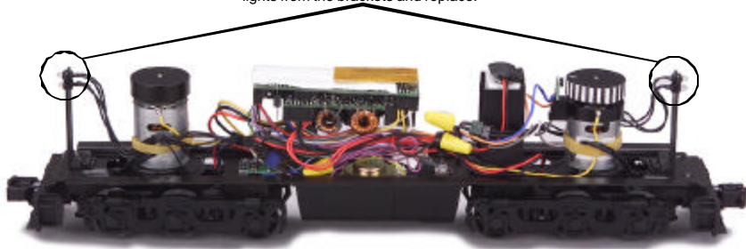
Figure 5. Location of the headlamp in the Engine.
