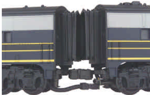
Figure 3: Connecting the Proto-Sound Harness
