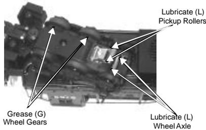
Figure 6: Lubricating The Locomotive Chassis
