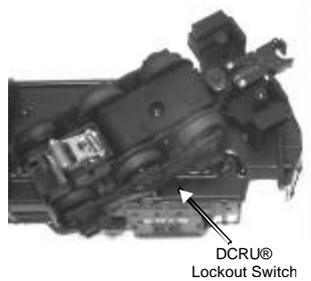
Figure 1: ProtoSound® DCRU® Lockout Switch
