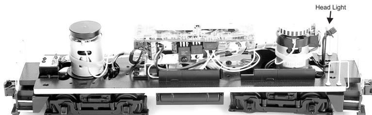
*Figure 4. Location of the headlamp in the Engine.*
