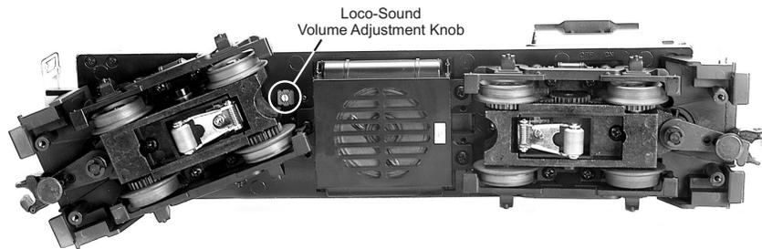
*Figure 1. Location of the Loco-Sound Volume Adjustment Knob*
