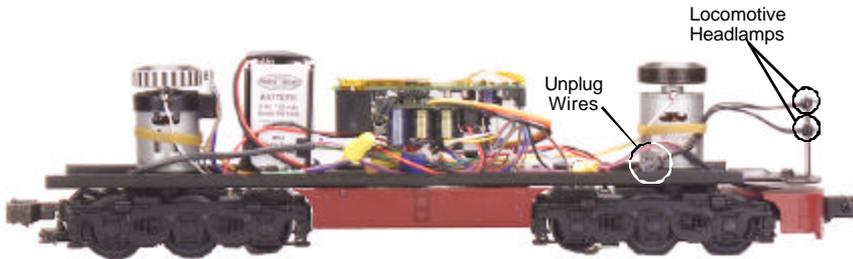
*Figure 5. Location of the headlamp in the Engine.*
