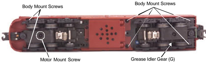
Figure 3. Body Mount Screws and Greasing Points.
