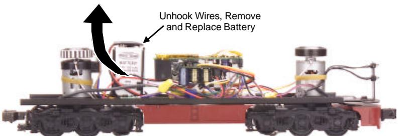
Figure 6. Removing and Replacing the Battery
