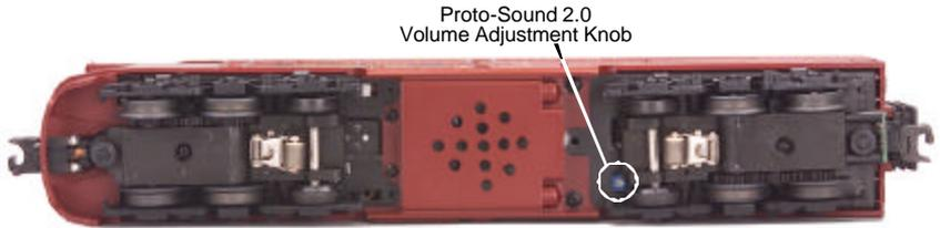
*Figure 1. Location of the Proto-Sound 2.0 Volume Adjustment Knob*
