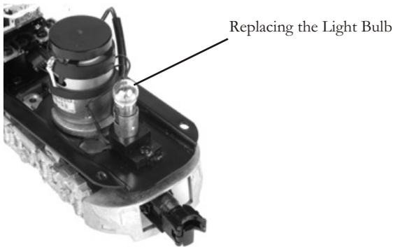
*Figure 5. Replacing the Light Bulb*
