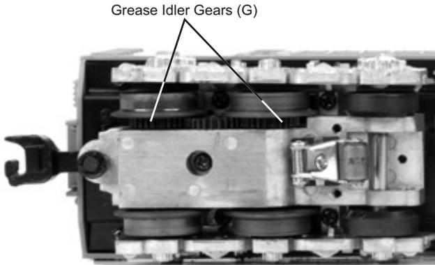
*Figure 4. Greasing The Idler Gears*
